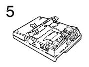
Insert the tabs of the wall mounting adaptor into the openings of the unit, then push it in the direction of the arrow. (The word "UP" on the adaptor should be upward.)
