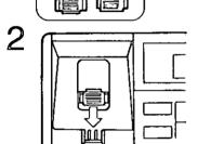
Replace the handset guide with making its tab upward.
