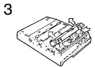
Remove the wall mounting adaptor from the bottom of the unit.
