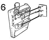
Connect the telephone line cord to the unit and to the wall-jack on the wall phone plate. Mount the unit on the wall phone plate, then seat securely by hooking as shown.
