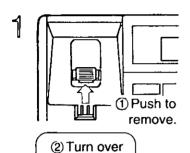
Remove the handset guide from the unit, then turn it over.
