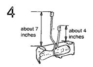
Tuck the telephone line cord inside the wall mounting adaptor.
